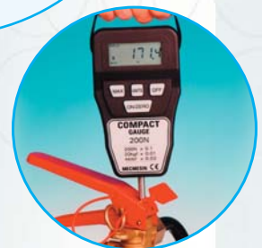
CFG Testing fire extinguisher
