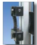
The ESM is shown in a typical tensile testing application, with Series BG digital force gauge, digital travel display, limit switch kit, and wedge grips
