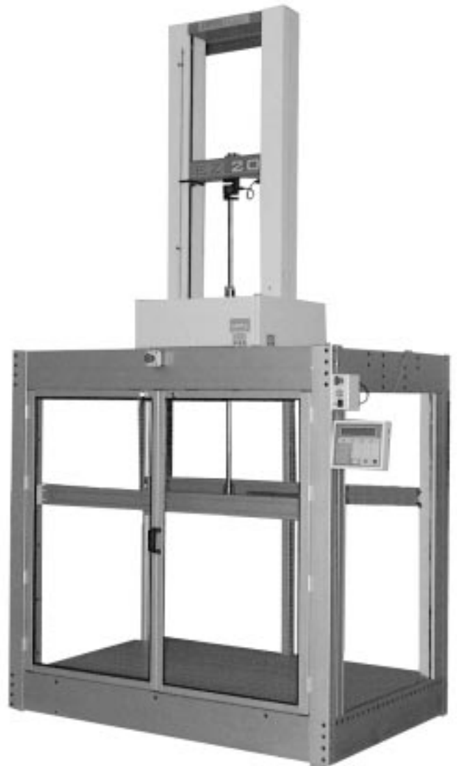
Cage size: 1300 mm (51.18 in) high x 1600 mm (62.99 in) wide x 1000 mm (39.37 in) deep
